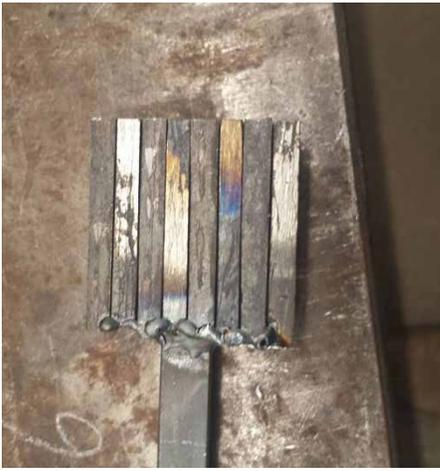
**Alternating stack of wrought iron and wrought steel**
